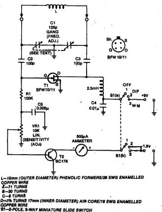
coil The plug-in forms are made from quality IV antenna connectors (male) and phenolic formers. latter, cut to 6cm lengths, are notched at one end to accommodate the connector, force fit and epoxied to Ceramic the former. connectors, available, should certainly be used instead.
