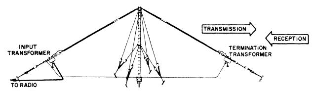
• The end of the HALF RHOMBIC ANTENNA with the TERMINATION TRANSFORMER points in the direction of BEST TRANSMISSION AND RECEPTION.
