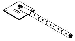
STEP 8 Slide the LOWER GUY PLATE (color code BLUE) onto the male end of the LOWER ADAPTER ASSEMBLY.
