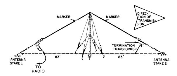
In the step-by-step procedure that follows, you will place two antenna stakes, each 83' away from the mast.
