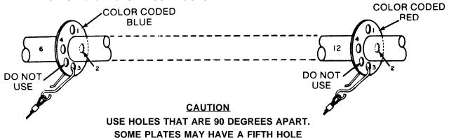
STEP 4 Attach each of the 4 GUY HOOKS (color code BLUE) to the proper hole on the LOWER GUY PLATE.
