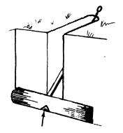
CUT AWAY SAPWOOD UNDER WASHER, SCREW NUT ON AS FAR AS IT WILL GO.
