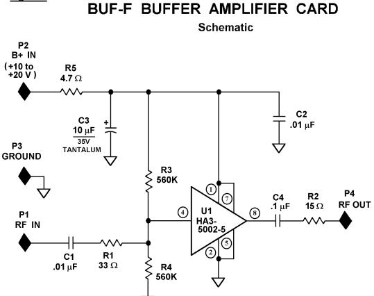
Figure 3 (above): BUF-F Amplifier Schematic (two per Switch / Amp. Box)
