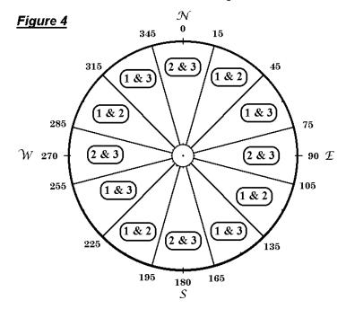
Loop Pairs to Use for Figure-of-8 Nulls in Specified Directions
