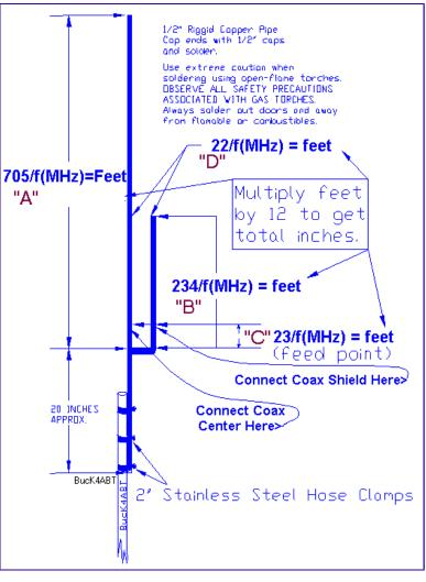
One is for 144 to 148 mHz (model JPOL2) and the other is for 430-450 mHz (model JPOL4).
