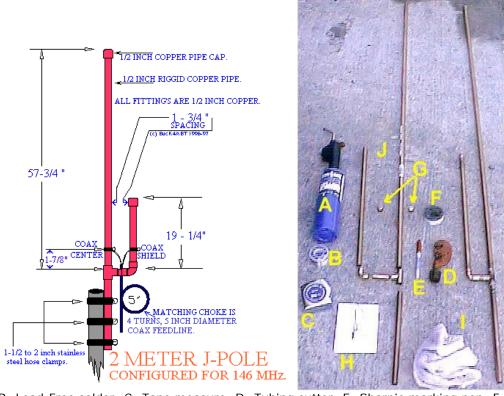
A=Benz-O-Matic propane torch; B=Lead-Free solder; C=Tape measure: D=Tubing cutter; E=Sharpie marking pen; F=Solder Paste; G=caps; H=Hardcopy of the above drawing; I=Wet Towel; J=PreCut, ready to assemble parts of the 2 meter J-Pole.
