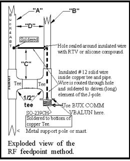
CLOSE UP of the alternative coax feed method. Use BUX VBALUN to couple coaxial cable to J-Pole.
